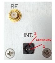
The majority of Isomet fused silica and quartz AO devices and high-power RF drivers are fitted with a 50degC switch. Refer to test data sheet.
